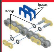
Included with every 520, 525 and 530 O-ring and Quadra-X Ring chain is a pair of spacers that help prevent damage to the sealing rings during installation of the connecting link. These spacers set the correct spacing between the inner and outer plates while riveting the connecting link, ensuring that the Orings seal properly and aren't under excessive pressure. Only EK Chain makes chain installation this easy.
